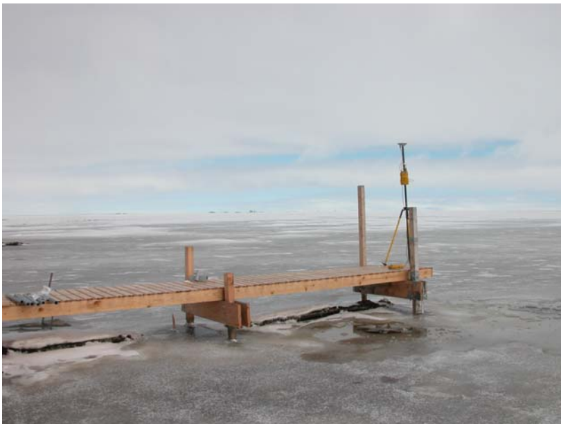
Dock on Cake Eater Lake installed in May 2006. A data logger is installed at the end of the dock in the upper water column and bottom sediments. The DGPS is seen positioned on the end of the dock ( photograph by Adrian Aguirre ).
