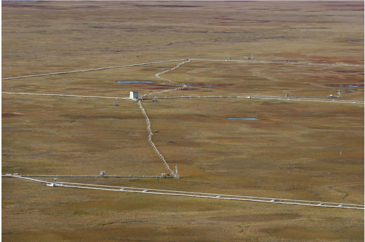
Figure 2. Aerial oblique photograph of the Biocomplexity site looking north. Boardwalks, trams, towers and instrument sheds were installed primarily in spring 2005 and 2006. In the foreground the south tram line closely parallels the boardwalk. A spur branches off and terminates at the southern most eddy tower. From the south tower (foreground), sampling tubes run north to the methane sampling shed (center), and the beginning of the north tram line. The boardwalk running west of the methane shed connects with the main boardwalk and runs north to south with access to all three trams and towers (left side). See Figure 1 for overall design.
